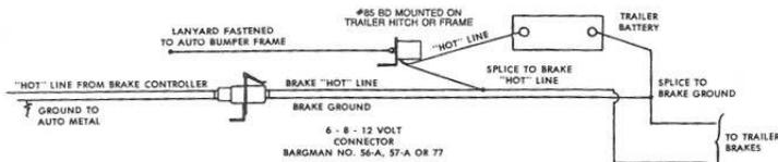
Keep trailer battery charged at all times to insure safe operation.
