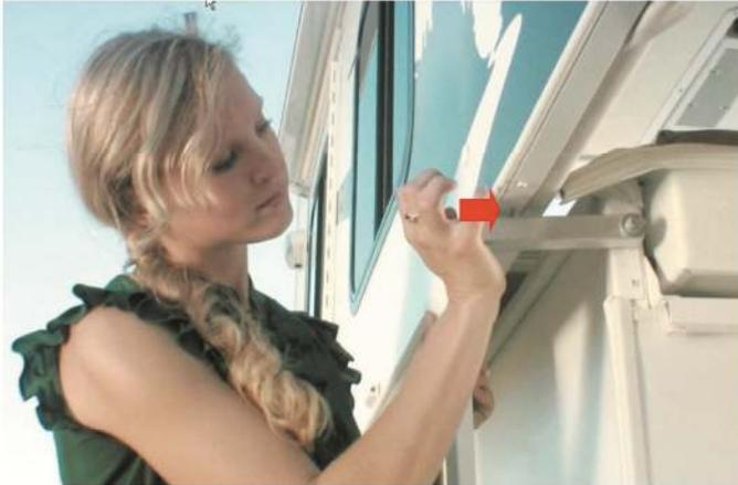
**Step 5:** Push the front corner latches onto the locking pins. For front slide models, after lifting the roof section and securing in place with the corner latches; grasp handle above gas bottles and pull living room section out toward you (or if your trailer is equipped with the electric slide option, operate the button to move the slide section out into position).
