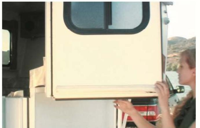
**Step 8:** Open top door section so it is against trailer wall.
