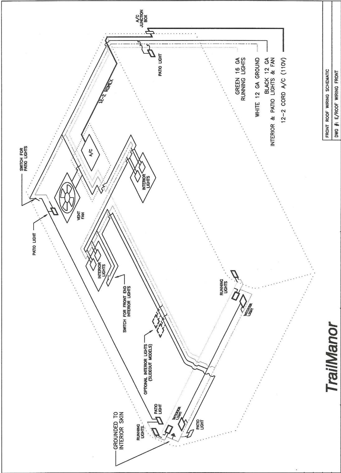
FRONT ROOF WIRING SCHEMATIC
