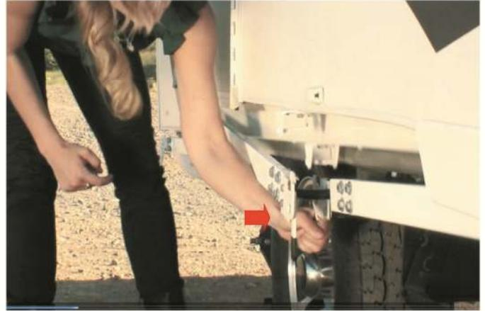
**Step 2:** Release the four black hold down latches, two on each side near the wheels.
