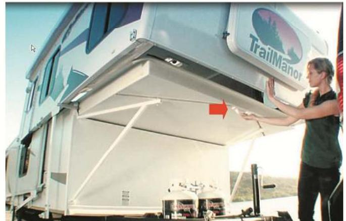
**Step 4:** Using the bed handle, pull out the bed until it stops.
