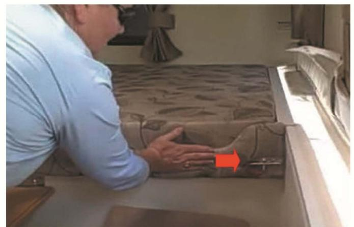
**Step 12:** Push mattresses out toward ends of trailer, and latch slide bolts BEFORE getting on bed. CAUTION: Bed can slip unless bolts are secured. On Slide out models, secure the slide bolts on the slide out once it is in place.
